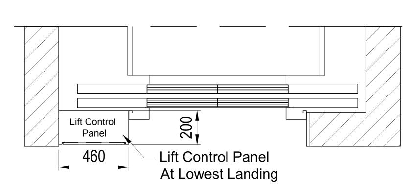
Lift Control Panel must be located at bottom floor only, next to the landing entrance
